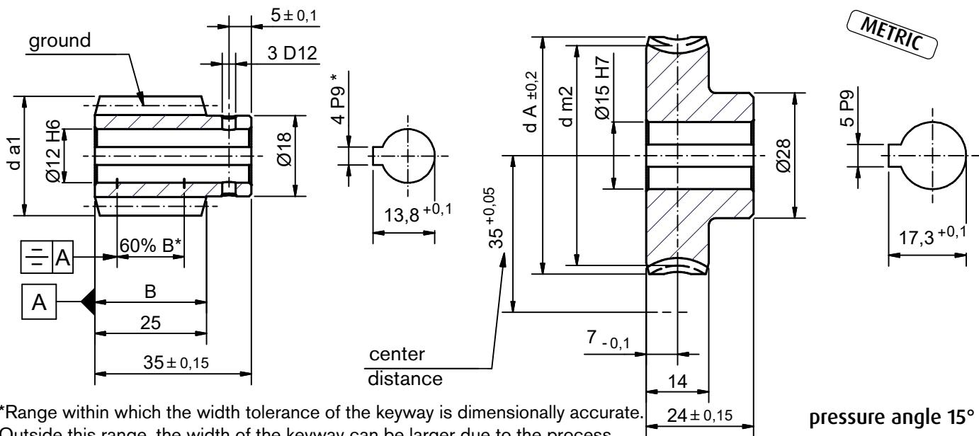
\*Range within which the width tolerance of the keyway is dimensionally accurate.
