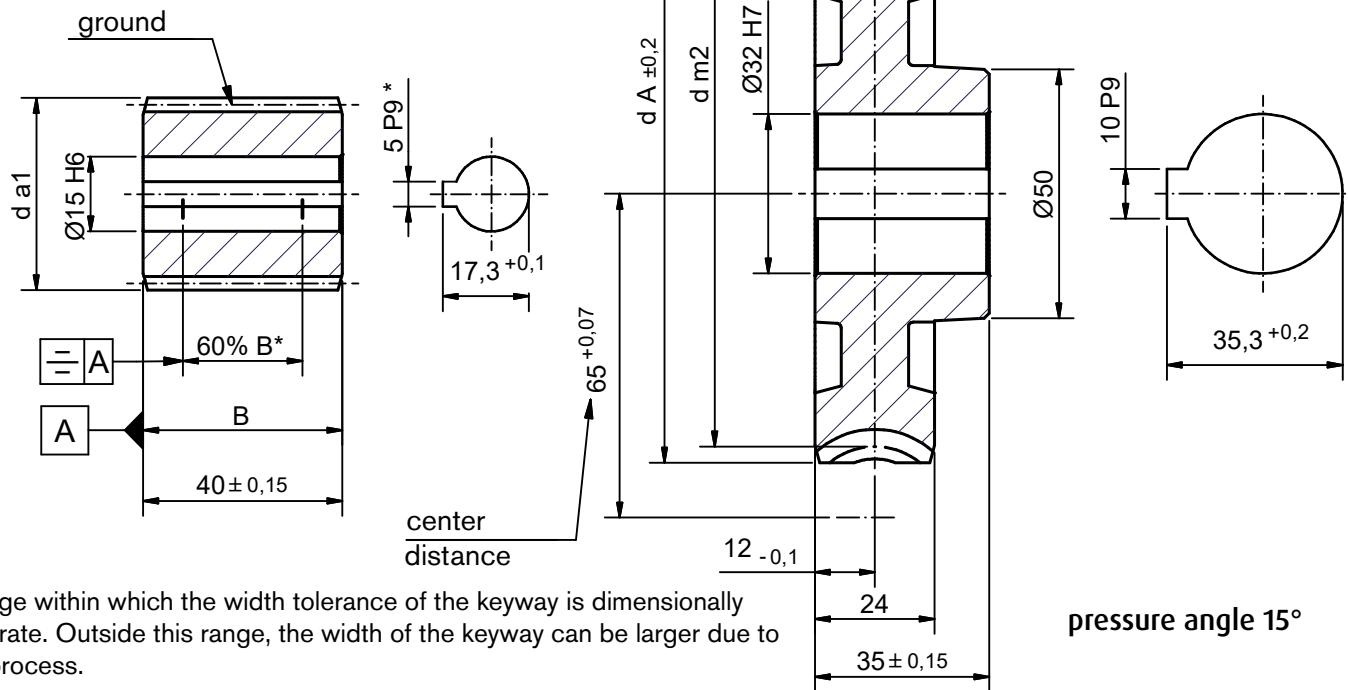
\*Range within which the width tolerance of the keyway is dimensionally accurate. Outside this range, the width of the keyway can be larger due to the process.
