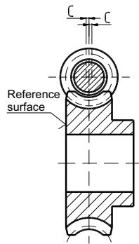
Use the reference surface for lateral adjustment. The lateral tolerance "c" must not exceed 0,15 mm regardless of the center distance.
