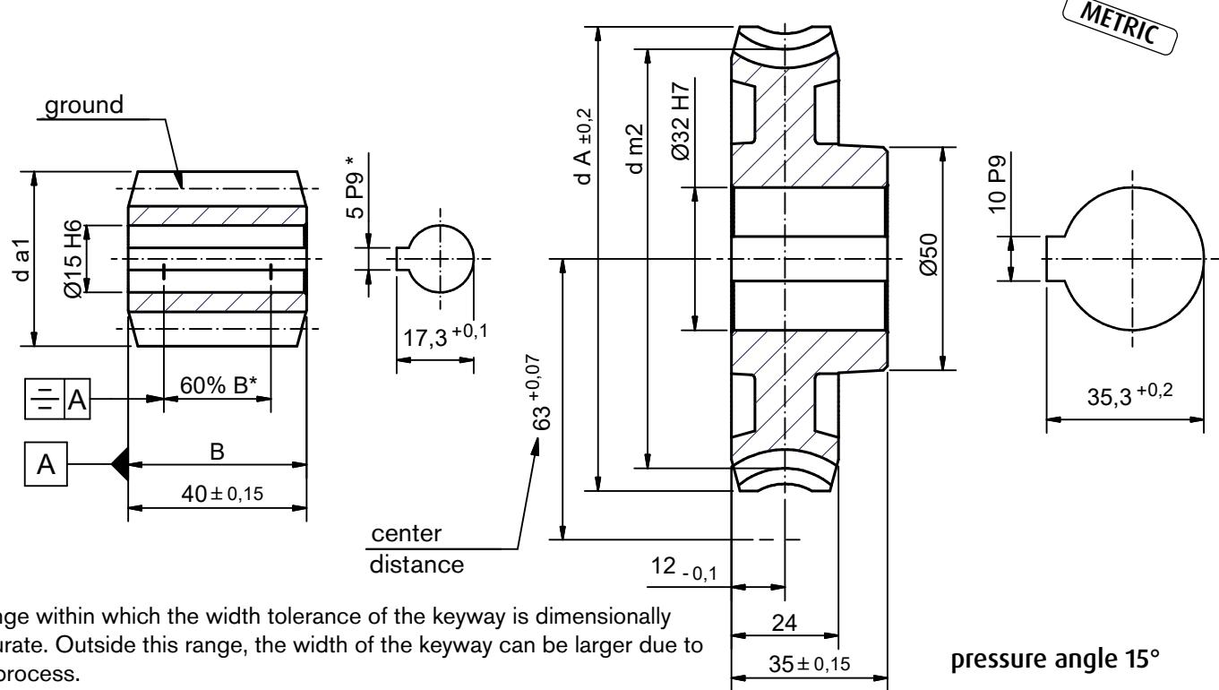
\*Range within which the width tolerance of the keyway is dimensionally accurate. Outside this range, the width of the keyway can be larger due to the process.
