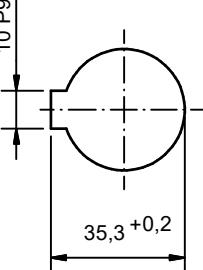
\*Range within which the width tolerance of the keyway is dimensionally accurate. Outside this range, the width of the keyway can be larger due to the process.
