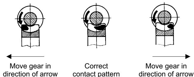
The contact pattern shows installation errors. The contact pattern should tend to the outgoing side. In case of reversing operation the contact pattern should tend to the center of the worm gear.
