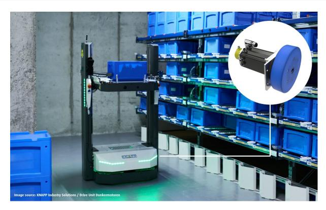
KNAPP's Open Shuttle is equipped with a combination of Framo Morat's NG500 hub gear and Dunkermotoren's BG 75 BLDC motor. (Image source: Knapp/Drive Unit: Dunkermotoren)
