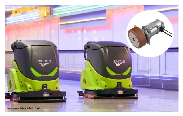
The ultra-compact and highly integrated RNA250 wheel hub drive from Framo Morat is used in the CR700 cleaning robot made by Adlatus. (Image source: Adlatus Robotics/Drive Unit: MinebeaMitsumi Technology Center Europe (MTCE) / Framo Morat)
