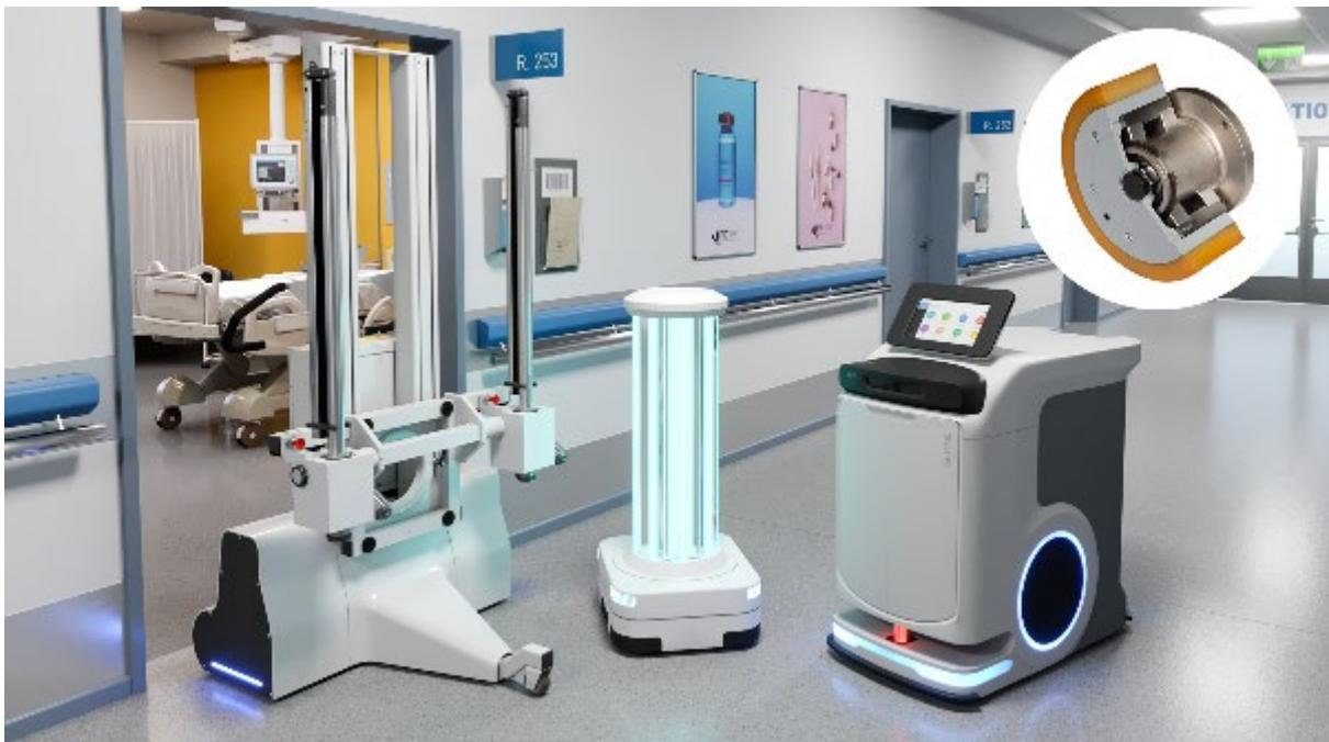
Wheel hub drives from the Framo Morat modular gearbox are used in various autonomous units such as disinfection robots and medical transportation vehicles – both in hospitals and in care facilities. (Image source: Franz Morat Group)
