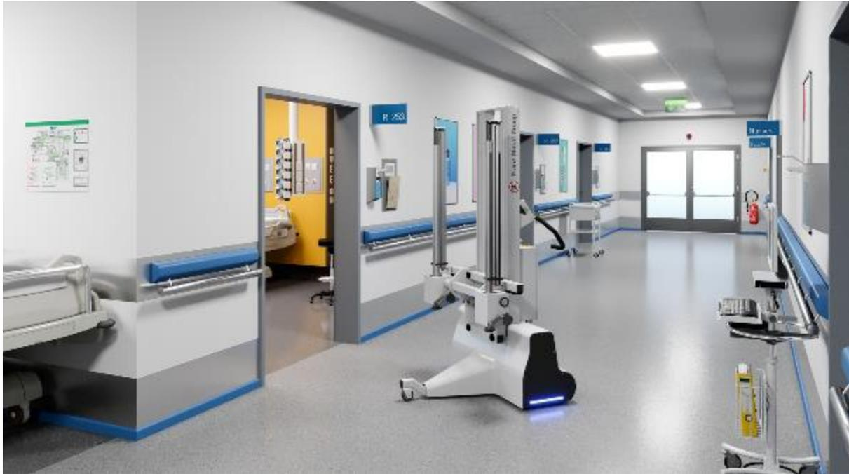
The system is available as an autonomously driven unit that can be navigated as needed to the desired location of use. (Image source: Franz Morat Group)
